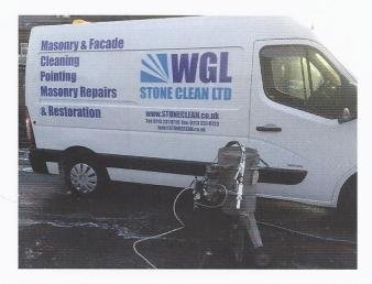
8. Earlier in 2018 and in response to customer demand, we purchased Stonehealth JOS/TORC stone polishing nozzle and abrasive pot set up. With JOS/TORC a light Calcium Carbonate abrasive forced through a vortex inducing nozzle that combines the abrasive with both air and water. JOS/TORC proves is ideal for light blasting applications stone damage to the substrate.
