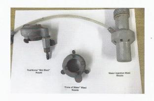
6. WE HAVE ALSO PURCHASED A SPECIAL NOZZLE FOR ABRASIVE GRIT BLASTING THAT INJECTS SMALL AMOUNTS OF WATER INTO THE AIR ABRASIVE MIXTURE TO CONTAIN DUST GENERATION.
