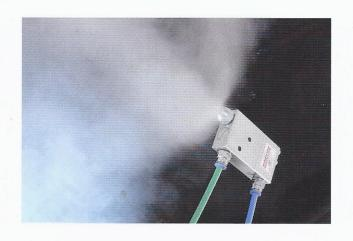
5. We developed an original cone shaped, water envelope when blasting in H.M. Prison, Armley. Rather than inject water into the air/abrasive stream the cone of water surrounds the abrasive stream totally eliminating the spread of dust while retaining the effectiveness of the dry blast stream.
